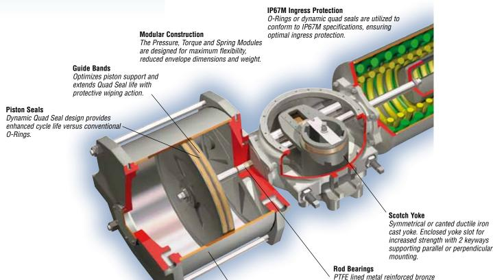
Heavy wall cylinders provide increased "job site" durability. Interior surface is honed and hard chrome plated to provide superior corrosion and wear resistance.
